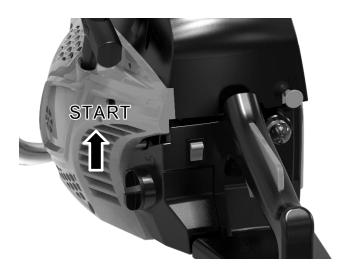
c. Pull the choke lever. It will close and the throttle will be moved to the starting position
