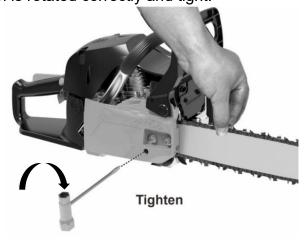
While lifting the chain guide, turn the content screw to apply correct tension to the chain.
