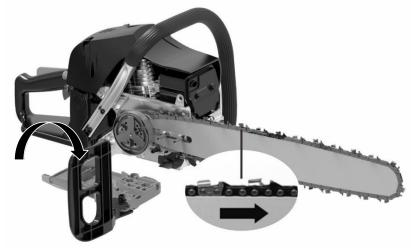
5) Attach the spiked bumper and screw it in place (if not installed).
